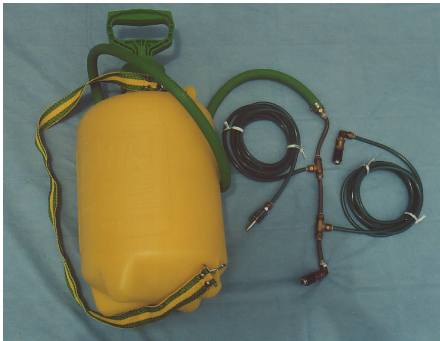
Umbilical lines to hookup water for three dental units.
